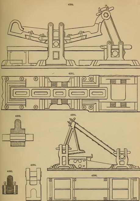
The squeezer has now almost entirely supplanted the hammer in the forge. Its first cost is not half so great, the cost of maintenance is diminished in a similar ratio, and if the quality of the iron
